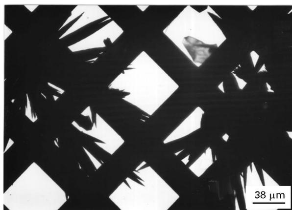
Figure 1 Aragonite imaged at low magnification on a TEM grid. The crystals develop from a common axis as needle-like.
